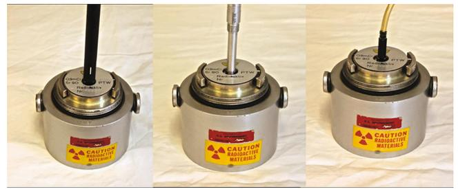
Fig. 1. Chamber placement in the  $^{90}\text{Sr}$  check source for the A12 chamber (left), IC69 chamber (center), and A28 chamber (right). Note that the A28 and IC69 chambers were inserted with the tip of the thimble resting on the bottom of the cavity, while the wider stem of the A12 chamber did not allow for the chamber to be inserted past the thimble.
