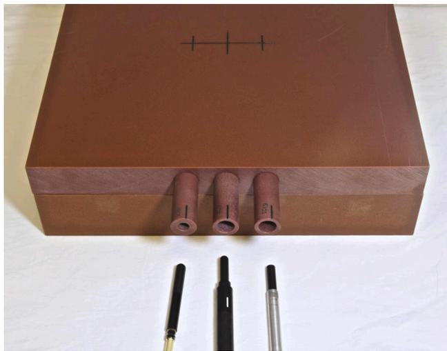
Fig. 2. Constancy Check Phantom (Standard Imaging, Middleton, WI) with chamber inserted and backscattering material. A 5 cm slab of Virtual Water™ was also added on top of the phantom shown for all measurements. The chamber location in front of the phantom indicates its location throughout all chamber stability trials.
